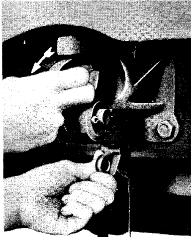
PRESS LATCH TO RELEASE JAW
