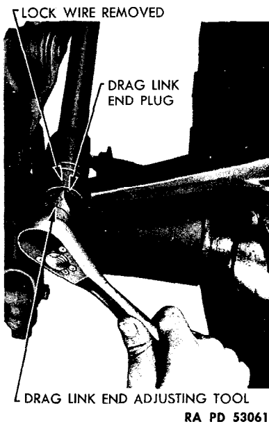
Figure 190—Adjusting Drag Link End
