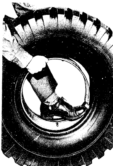
EXPANDING TIRE BEAD LOCK RING IN TIRE
