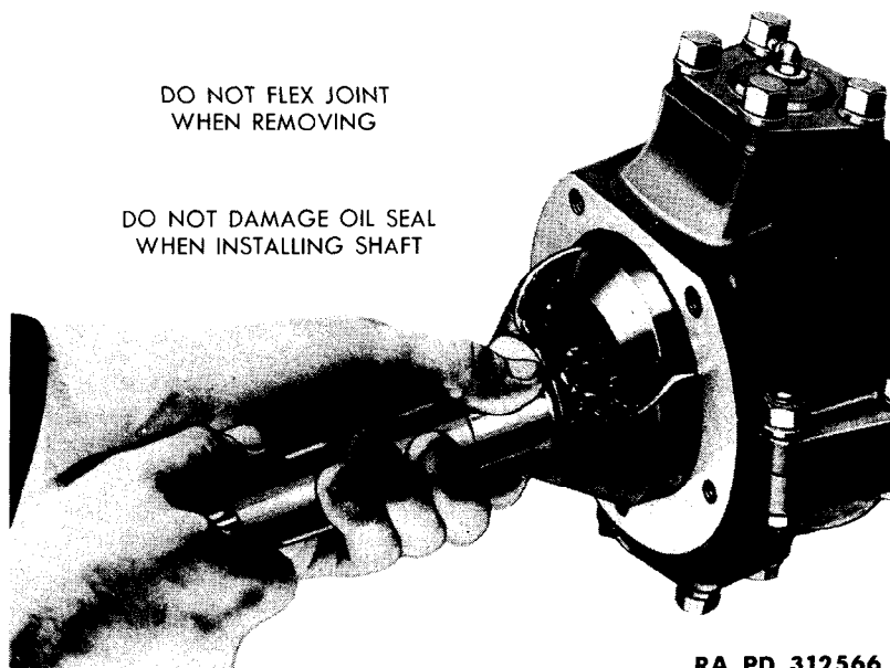
Figure 157—Removing Universal Drive Assembly
